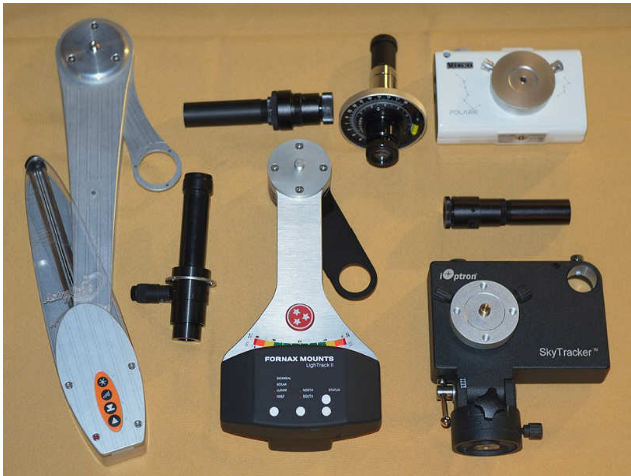
Figure 8.1.0.1A. Popular past and present tracking mounts. The left two have good payload capacity. The four tracking mounts shown here are reviewed or otherwise noted. These are: * LEFT: AstroTrac TT320x star tracker. Optional polar alignment scope immediately to its right. * CENTER: Fornax LightTrack II mount. Optional CG5 polar alignment scope is to its upper left. * UPPER RIGHT: Vixen Polaris tracker. Its optional polar alignment scope is just to its left. * LOWER RIGHT: iOptron SkyTracker. Its included polar alignment scope is just above it.
