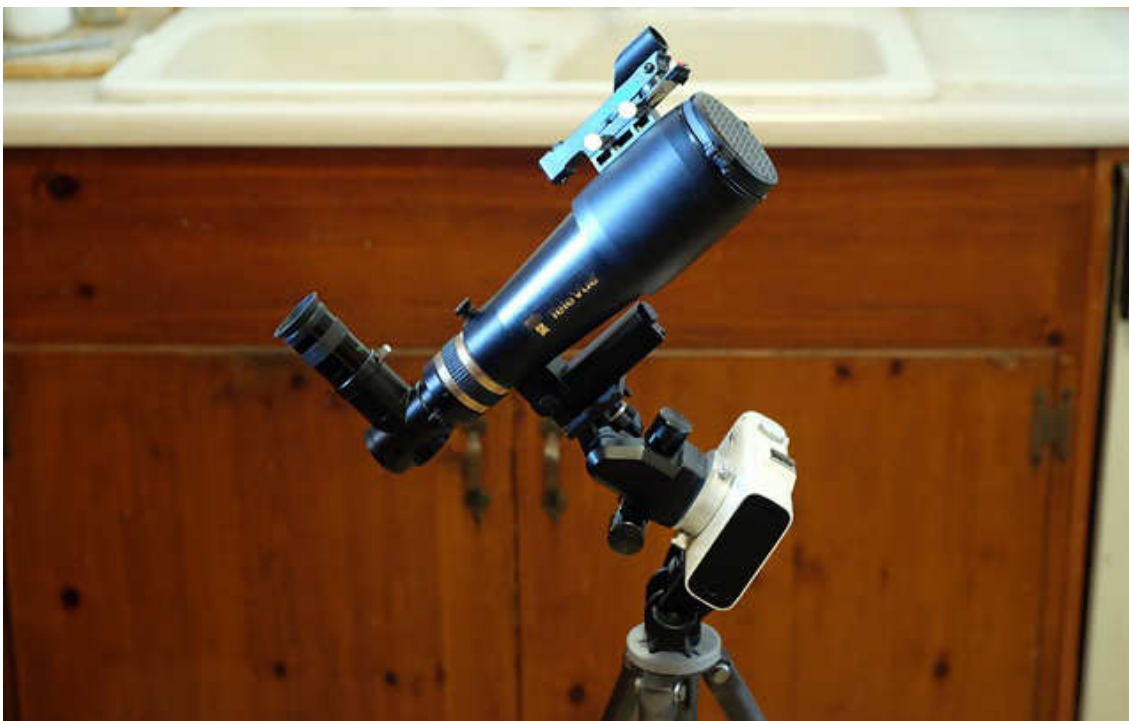
Fig. 3.5A. Compact TeleVue 60 ED refractor telescope, shown mounted on a Vixen Polaris star tracker. I use a flip cap on the front to minimize time that the objective lens is exposed to the elements.
