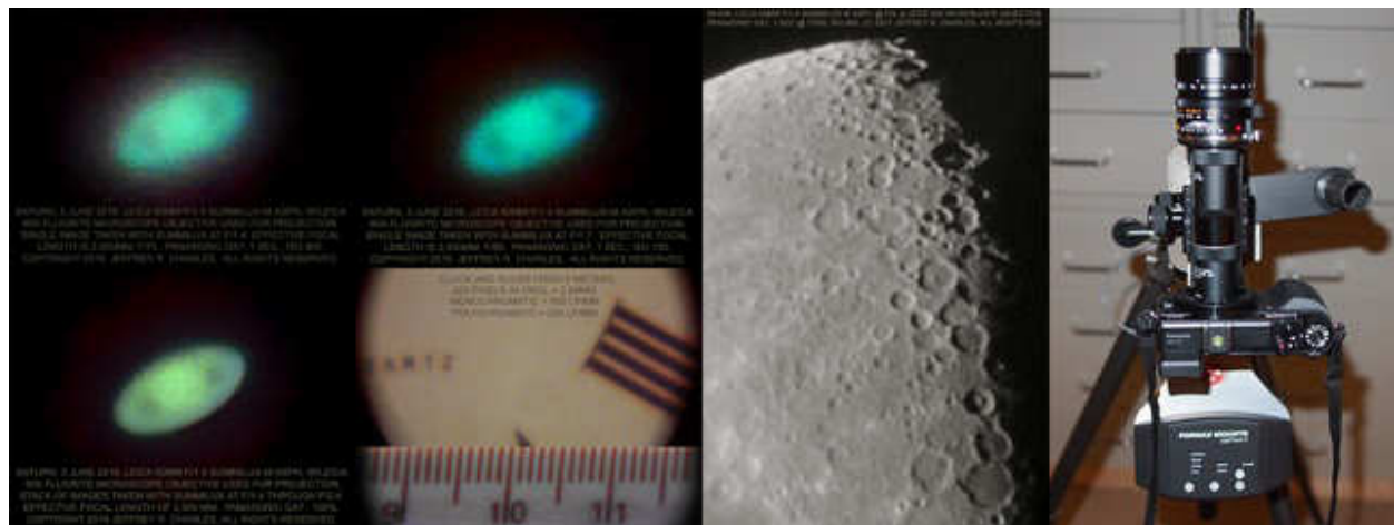
Figure 3.2A. Saturn and moon, using Leica 50 mm Summilux lens as a “telescope objective”. LEFT: These cropped images of Saturn were taken with a Leica 50 mm FL f/1.4 Summilux-M ASPH lens. A microscope objective and extension tubes were used behind the lens to provide an effective focal length of about 2.500 mm. The Leica lens was used at full aperture for the upper left image, and at f/1.7 for the image just to its right. The lower left image is a stack of about 3 images. The photo just right of the stacked image is of a ruler (millimeter scale), imaged from a distance of 5 meters with the same optics. RIGHT: Moon, with same optics that were used for Saturn images. The extreme right image shows a Panasonic GX7 camera attached to the setup.
