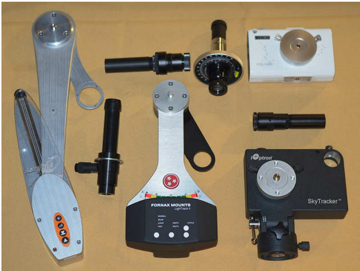
Figure 8.1.0.1A. Popular past and present tracking mounts. The left two have good payload capacity. The four tracking mounts shown here are reviewed or otherwise noted. These are: * LEFT: AstroTrac TT320x star tracker. Optional polar alignment scope immediately to its right. * CENTER: Fornax LighTrack II mount. Optional CG5 polar alignment scope is to its upper left. * UPPER RIGHT: Vixen Polarie tracker. Its optional polar alignment scope is just to its left. * LOWER RIGHT: iOptron SkyTracker. Its included polar alignment scope is just above it.
