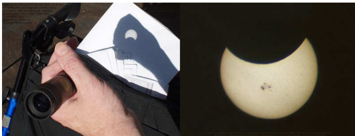
Figure 3.1A. Projecting a partial solar eclipse via monocular; photo of projected eclipse image. LEFT: On 23 Oct 2014, a partial solar eclipse was in progress when I arrived at work. The eclipse happened while a large sunspot group was visible, so it was more dramatic than most partials. Here, the Specwell 8 x 20 monocular is used to project an image of the eclipse onto some paper that is used as an impromptu projection screen on my walker. The monocular is held in a way that my hand shades the projection “screen” around the image. RIGHT: Close up photo of projected image that is rotated and flipped to approximate the orientation of the eclipse in the sky. There is some distortion of the sun’s circular shape due to the angle of the projection versus the camera position, but it is far better than having no picture at all of this memorable event. A few passers by stopped to look at the projection during the brief time it took to take this picture.
