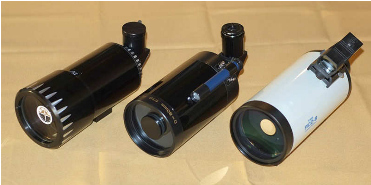
Figure 3B. Three small amateur telescopes of similar aperture that were made in different eras. Unfortunately, quality has declined over the years. From left to right, the pictured telescopes are: * Ad Astra III, a high quality 7.8 cm Maksutov-Cassegrain telescope from the late 1970's. * Bausch & Lomb 800, a low cost hybrid Cassegrain mirror camera lens and telescope from the 1990's. Finder scope is custom addition. Standard telescope does not have a finder scope or a way to attach one. * Kasai Pico-8, a disappointingly awful Maksutov-Cassegrain telescope I acquired new in 2018. In general, a telescope performs better than a camera lens that is used as a telescope, but this one does not.
