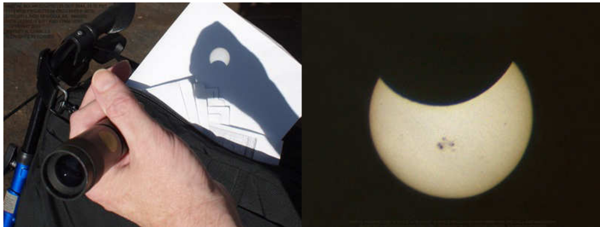
Figure 3.1A. Projecting a partial solar eclipse via monocular; photo of projected eclipse image. LEFT: On 23 October, 2014, a partial solar eclipse was in progress when I arrived at work. The eclipse happened while a large sunspot group was visible, so it was more dramatic than most partials. Here, the Specwell 8 x 20 monocular is used to project an image of the eclipse onto some paper that is used as an impromptu projection screen on my walker. The monocular is held in a way that my hand shades the projection “screen” around the image. RIGHT: Close up photo of projected image that is rotated and flipped to approximate the orientation of the eclipse in the sky. There is some distortion of the sun's circular shape due to the angle of the projection versus the camera position, but it is far better than having no picture at all of this memorable event. A few passers by stopped to look at the projection during the brief time needed to take this picture.
