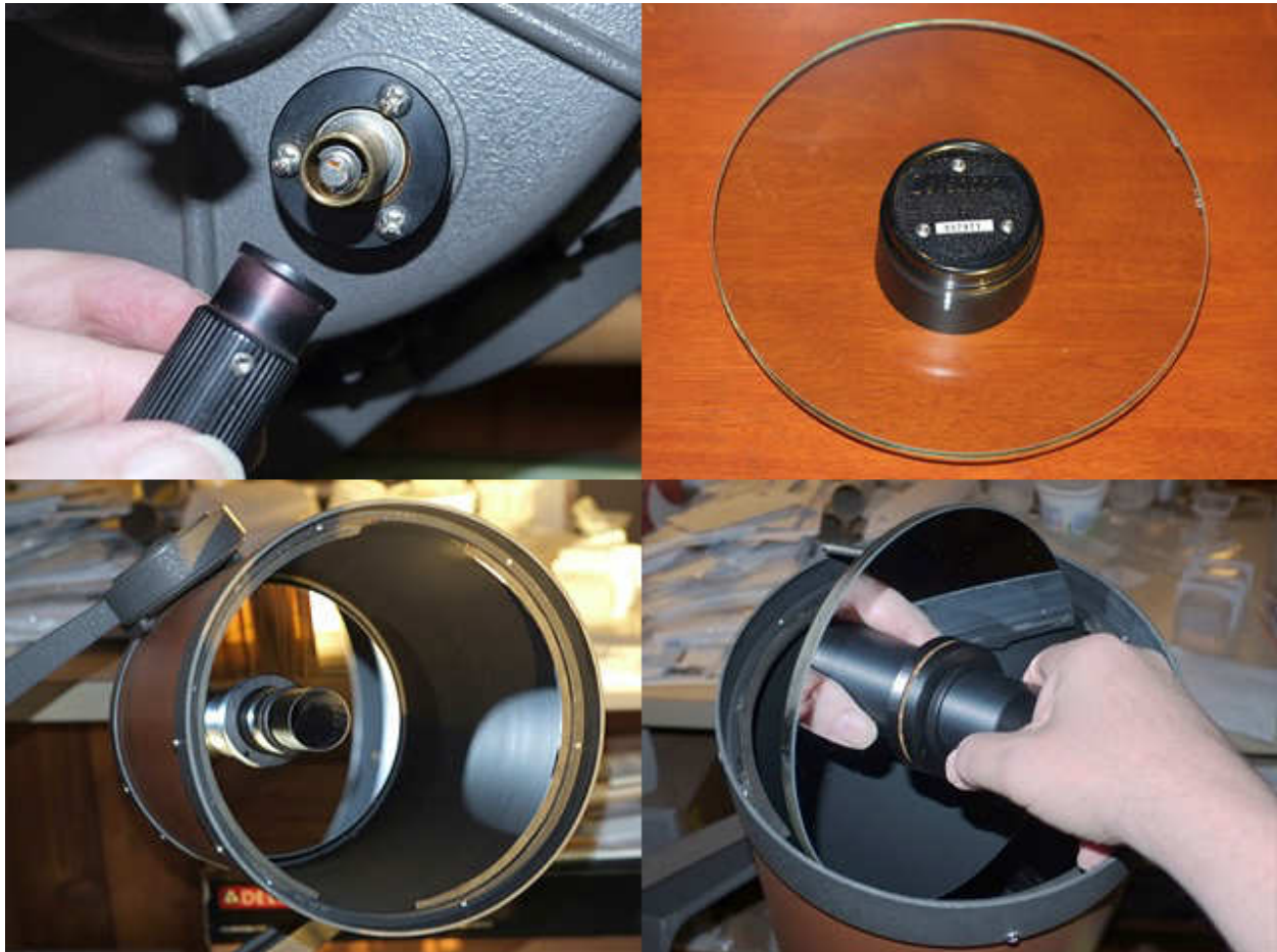
Figure 9.2.2.1A. Servicing a Celestron 8 SCT: Photos of some of the steps described below. UPPER LEFT: Preparing the focus mechanism, to facilitate later removal of primary mirror. A retaining screw or ring (depending on model) must be removed from the end of the focus bolt that is visible inside the brass fitting on the telescope. This version uses a retaining ring. UPPER RIGHT: Schmidt corrector plate removed, set in safe place. A cover is recommended. LOWER LEFT: C8 OTA with corrector plate removed. Primary mirror removal slots are at the top and bottom of the photo for this model. C-ring around primary baffle tube must be removed. LOWER RIGHT: Removing the primary mirror by tilting it so it will fit through the mirror removal slots in the front cell, without marring the mirror coating. Take care to keep the mirror edge from hitting the cell or baffle tube, since this can cause chips. The OTA is pointed vertical for this step. The focus bolt is toward the upper left of the photo, sticking out behind the mirror.
